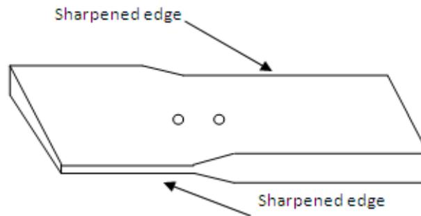
Figure 2: The cutting blade
